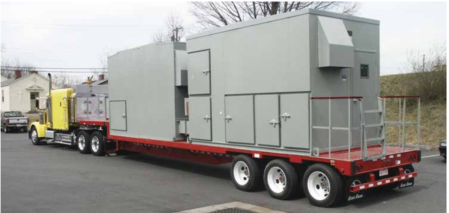
Totally-Enclosed Portable Substation with Heavy Insulation for Extreme Cold Environment
