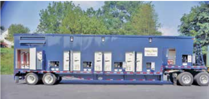
Dual-Rated 12.47 and 24.9 kV Portable Substation
